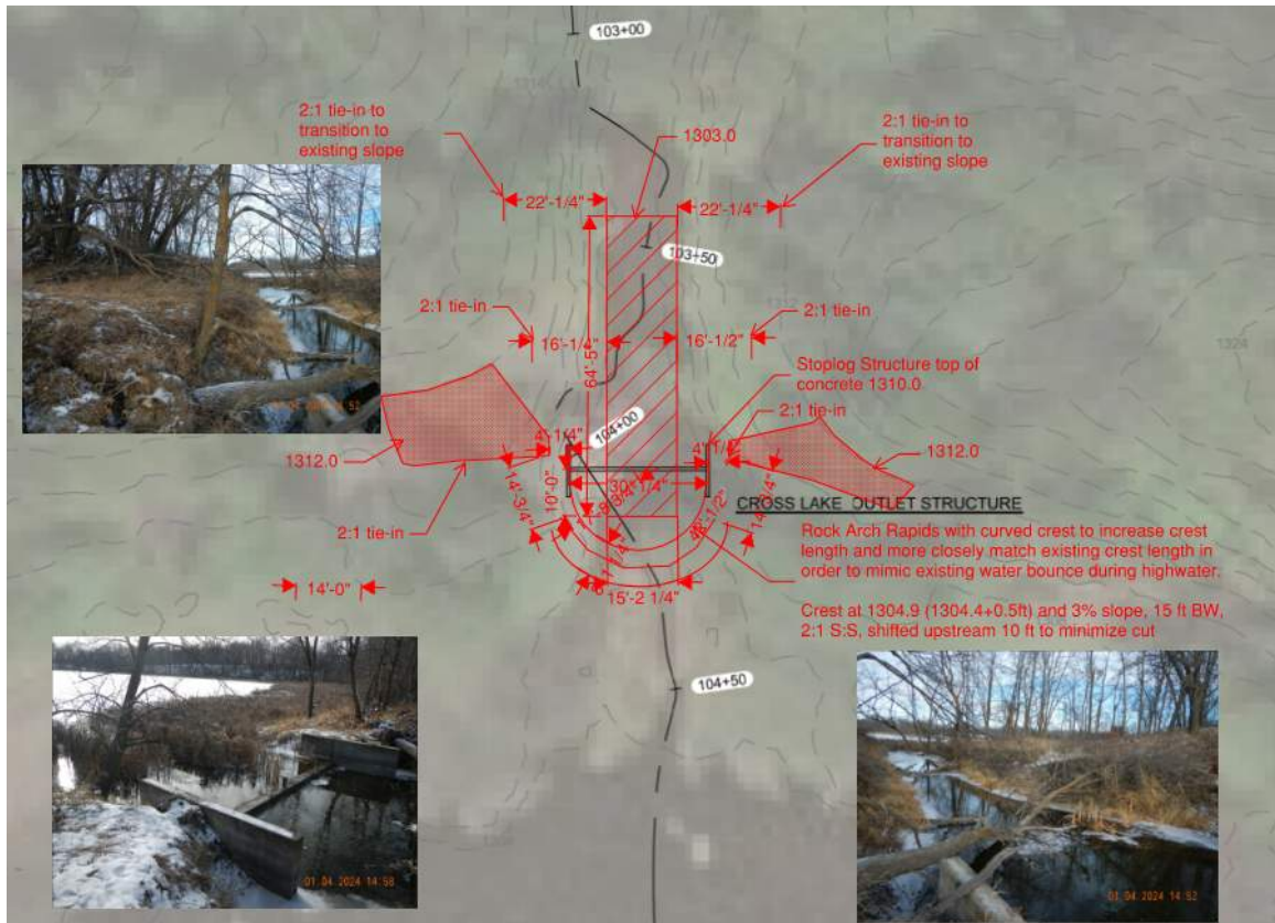
Figure 12: Example Cross Lake Outlet Structure Layout Considered During the Feasibility Study
